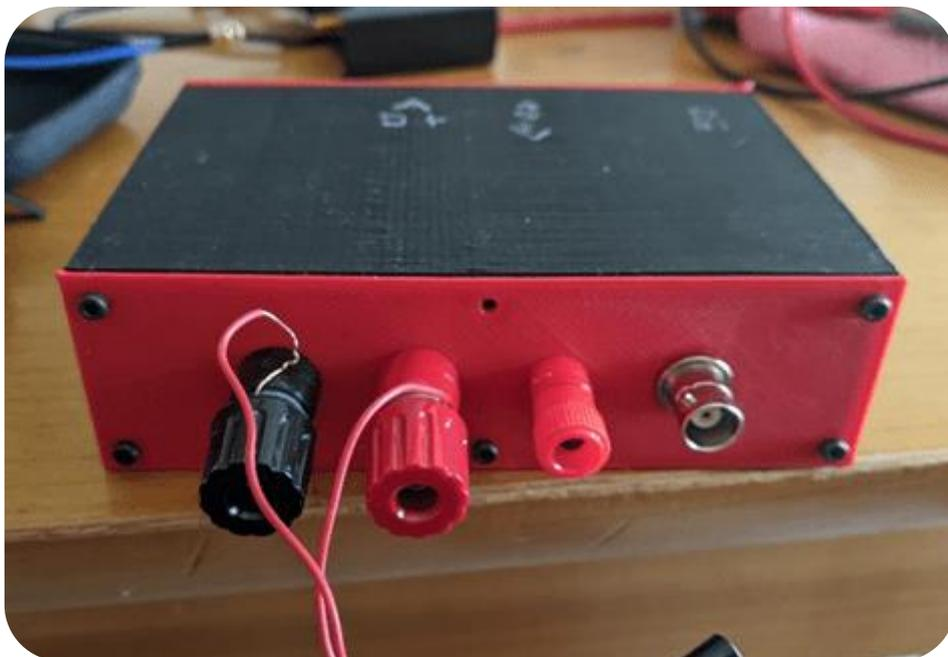
FIGURA 3 RETRO CON USCITA A BASSA ED ALTA IMPEDENZA
