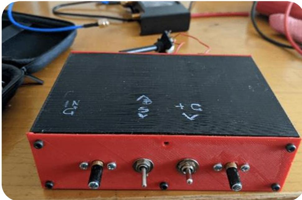
FIGURA 4 FRONTE. UN SELETTORE INSERISCE DELLA CAPACITÀ IN INGRESSO, SE NECESSARIO. IL SECONDO
